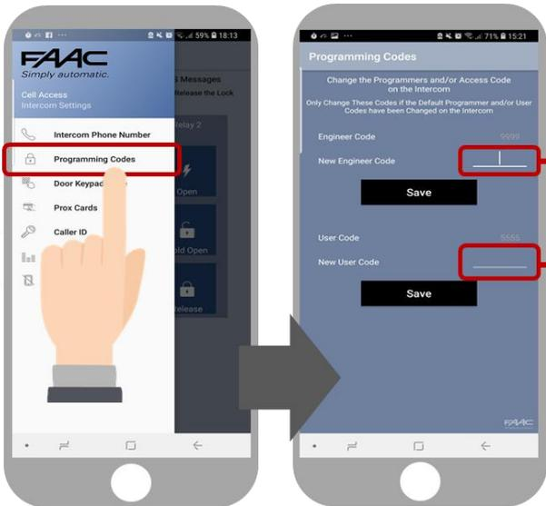
Enter 9999 (unless changed by engineer on the intercom) and press SAVE
