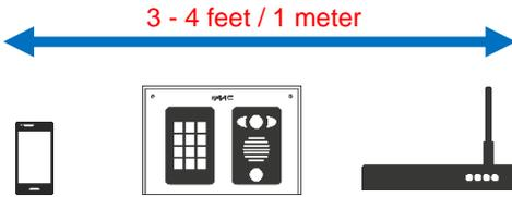
Do not install the intercom. Power it up beside the router so that you can perform the configuration with the homeowners' phone beside the intercom and router.
