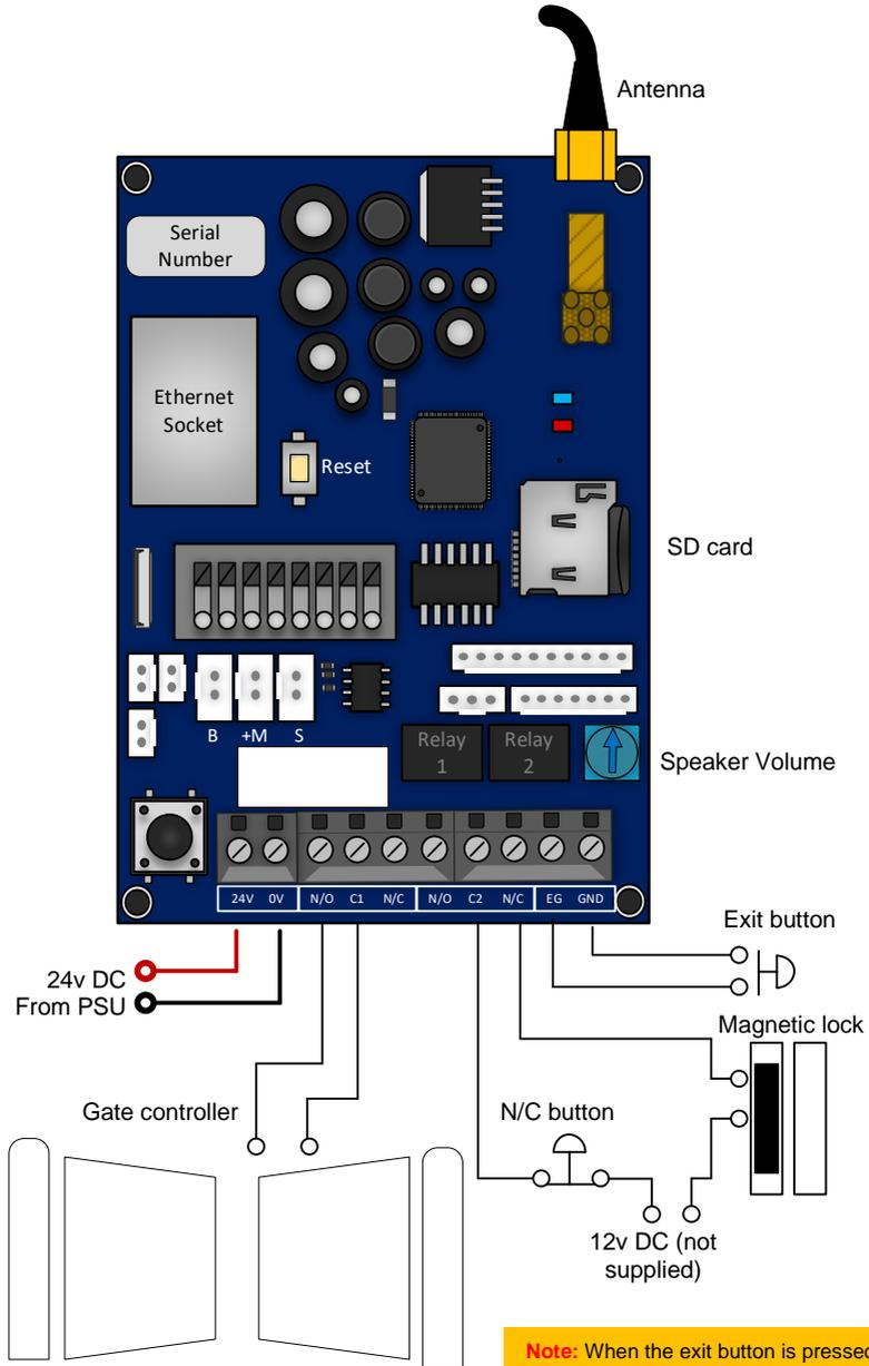
**Note:** When the exit button is pressed it will trigger relay 1 for the pre-programmed time in the app. (Default is 1 second)
