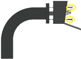
Use the pre-drilled mounting holes and cable cut outs to connect the intercom to the mounting option chosen.
