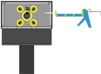
Seal all mounting or cable cut outs by using sealant such as silicone.
