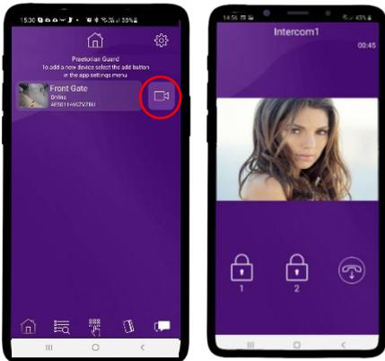
**Note:** If you can see live video and hear audio, the intercom has successfully connected to the network. If for some reason this does not work, check the LED indicators on the RJ45 socket on the PCB to ensure it is connected correctly to the network.
